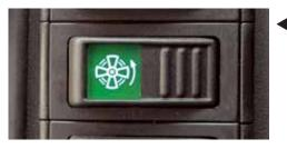
Intelligent ECO Fan\* for better efficiency. The angle of the vanes on the fan changes depending on the operating temperature in order to save fuel consumption. Alternating the direction of air flow cleans the heat exchanger automatically.
