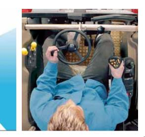
The sloping hood, "A" post-mounted exhaust, sculpted body and full length glazed doors put the working area in your field of vision. The CVX also has a roof window: ideal for loader work. Multicontroller IV puts all the tractor's key functions in the palm of your hand for maximum comfort.
