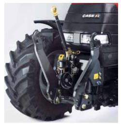
A front-PTO\* and front-mounted hitch\* with a maximum lift capacity of up to 4,000 kg is available to give your CVX more versatility.
