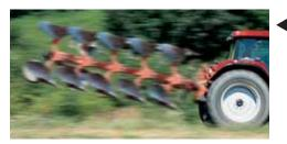
The fully integrated hitch ride control feature with Bosch-EHC (Electronic Hitch Control) neutralises any vibrations caused by heavy implements when travelling at high road speeds for extra comfort and safety.
