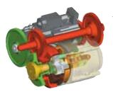
The summation planetary set combines the mechanical and flexible hydrostatic power transmission into continuous, smooth movement.
